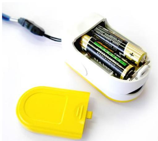
Figure 3. Batteries Installation
